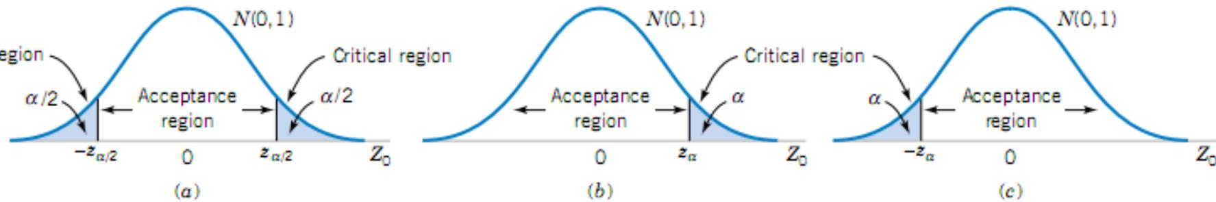
**Figure 9-6** The distribution of  $Z_0$  when  $H_0: \mu = \mu_0$  is true, with critical region for (a) the two-sided alternative  $H_1: \mu \neq \mu_0$ , (b) the one-sided alternative  $H_1: \mu > \mu_0$ , and (c) the one-sided alternative  $H_1: \mu < \mu_0$ .
