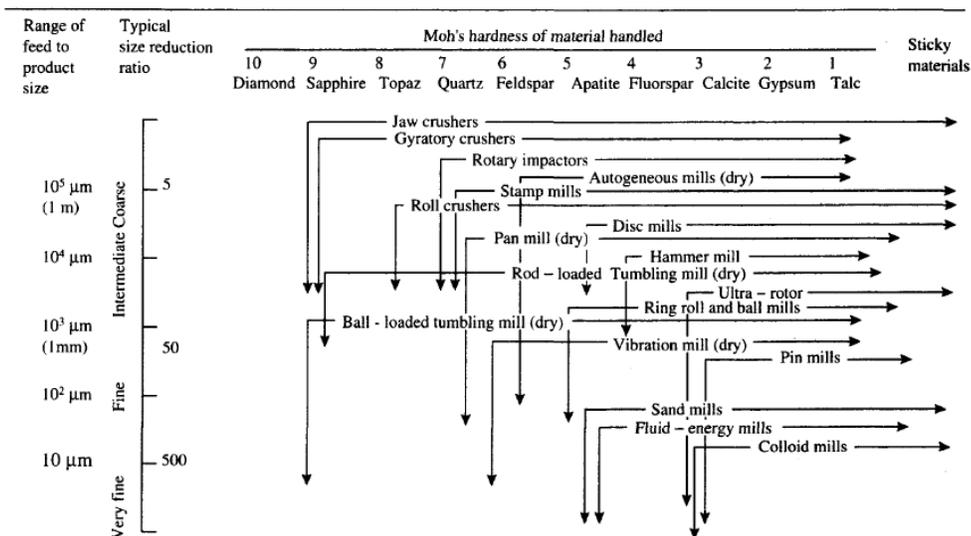
Table 10.13. Selection of comminution equipment for various materials (after Marshall, 1974) Note: Moh's scale of hardness is given in Table 10.12
