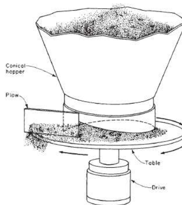
FIG. 21-29 Table feeder. The skirt is raised in a spiral pattern for increased capacity in the direction of rotation. (Courtesy of Chemical Engineering.)
